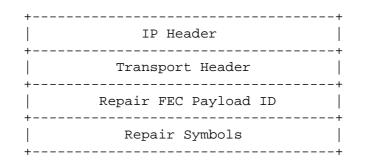
Figure 7: Packet Format for FEC Repair Packets
